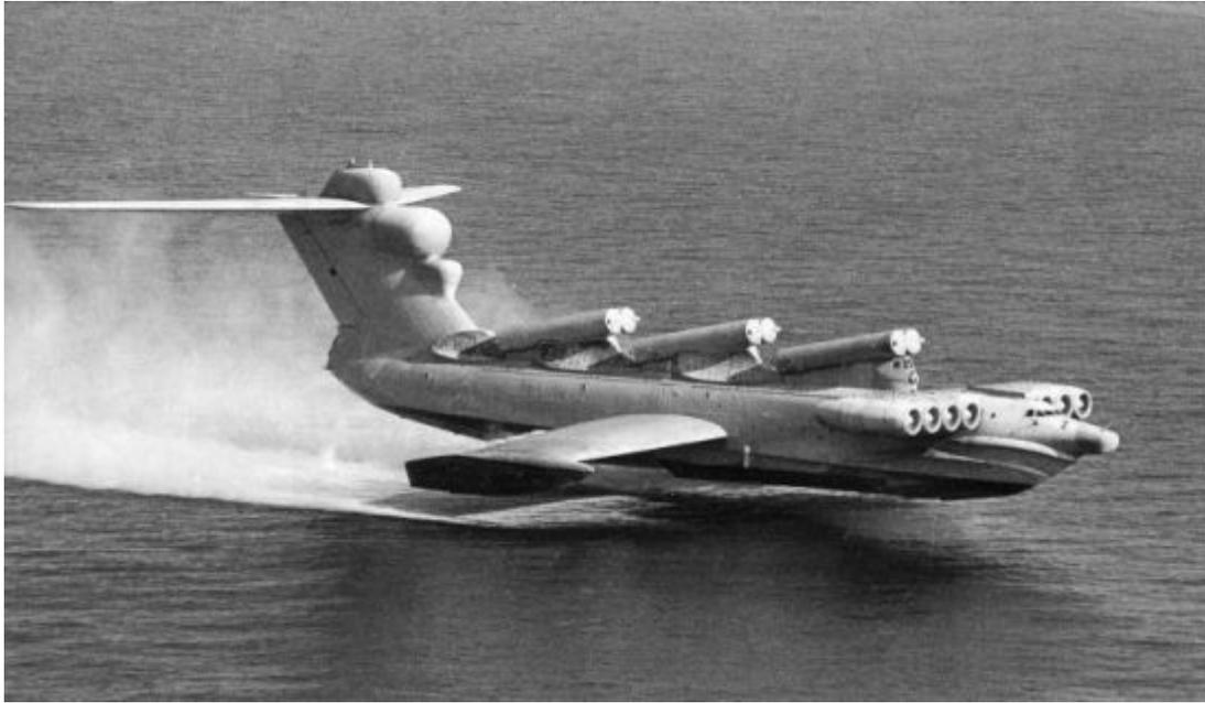
**Lun Ekranoplan with missile launchers mounted above the fuselage**
