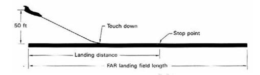
A sketch depicting the FAR landing field length is shown in figure H.1. The landing field length as defined in figure H.1 usually appears in specifications for transport aircraft designed to the criteria of FAR part 25
