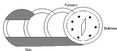
2. > Semi-Monocoque construction → Constructed of alloys of Al, Mg although steel and titanium are also used in area of high temperature. This construction uses
