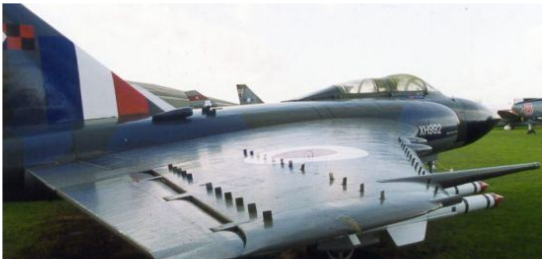
A Gloster Javelin showing the three sets of vortex generators located along the outer portion of the wing
