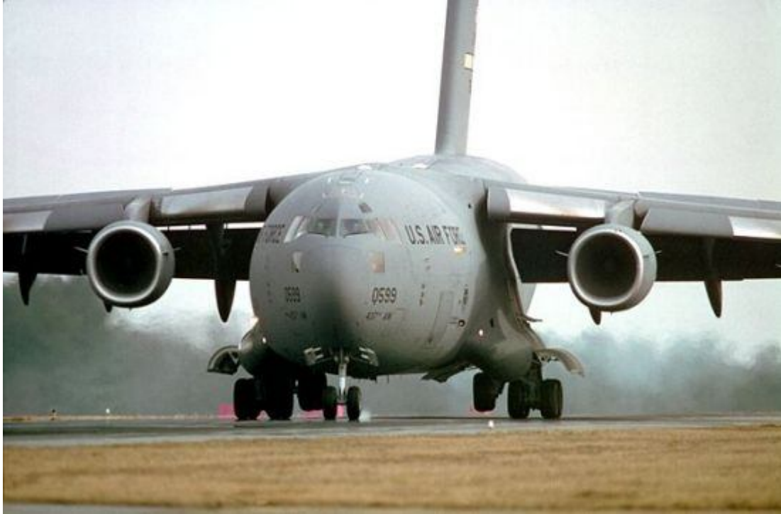
Large vortex generator plates visible on the engine cowlings of a C-17
