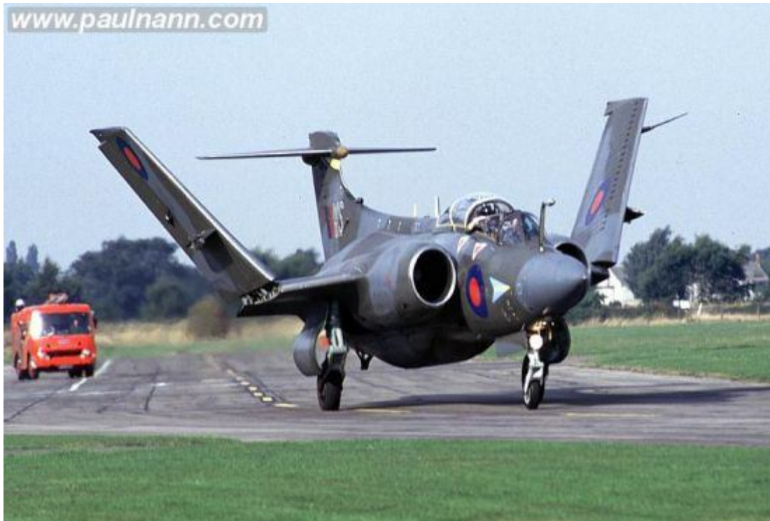
A Buccaneer folding its wings, note the vortex generators near the leading edge
