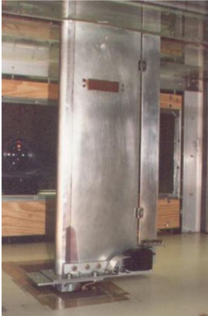
2D infinite wing being tested in a wind tunnel
