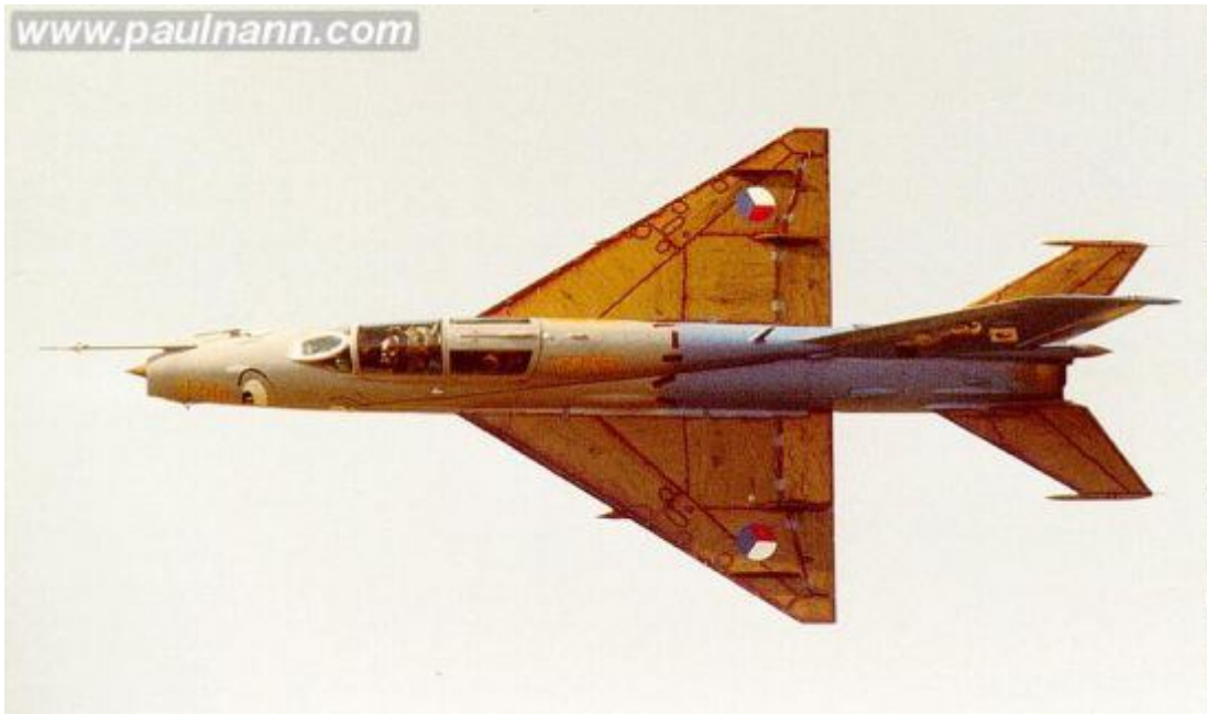
MiG-21 fighter showing its low aspect ratio wing
