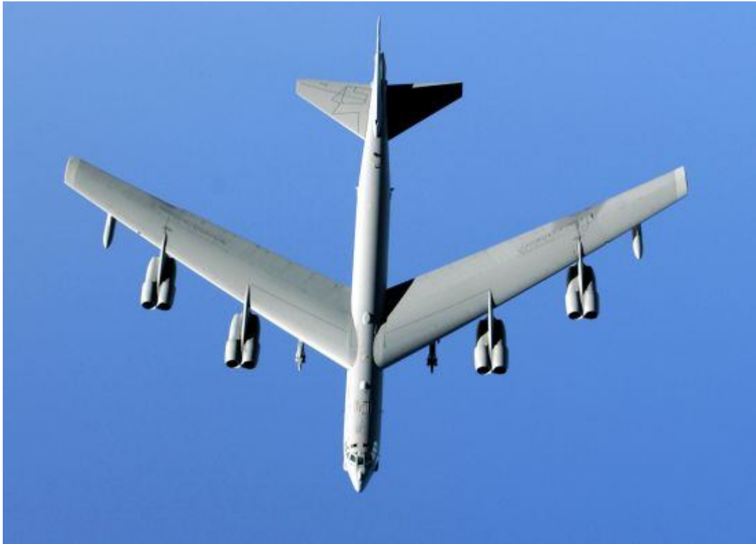
Overhead view of a B-52 illustrating its high aspect ratio wing
