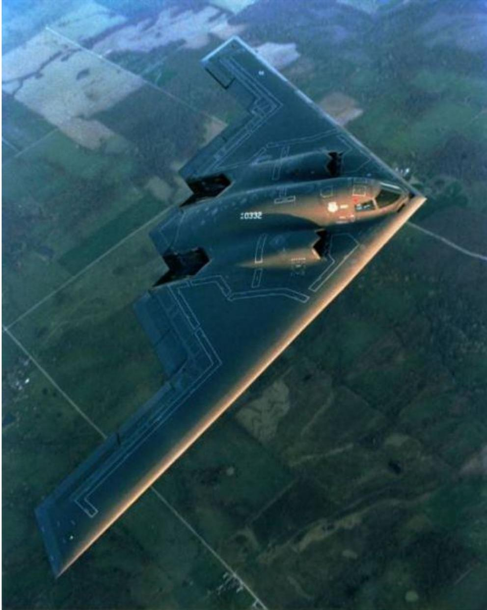
**Overhead view of the B-2 stealth bomber showing its long nozzle troughs**
