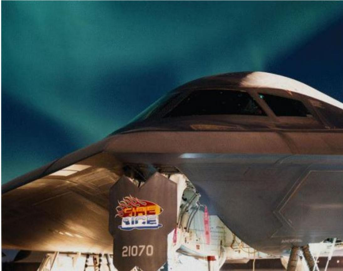
**Saw-toothed edges used on the B-2 Spirit nose landing gear door**
