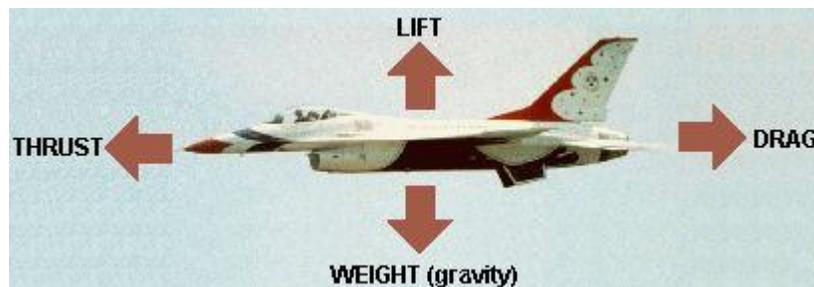
**Four forces acting on an aircraft in flight**
