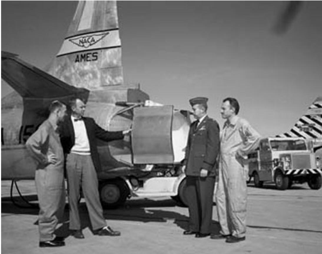
**Thrust reverser used on the F-94C during NASA experiments**
