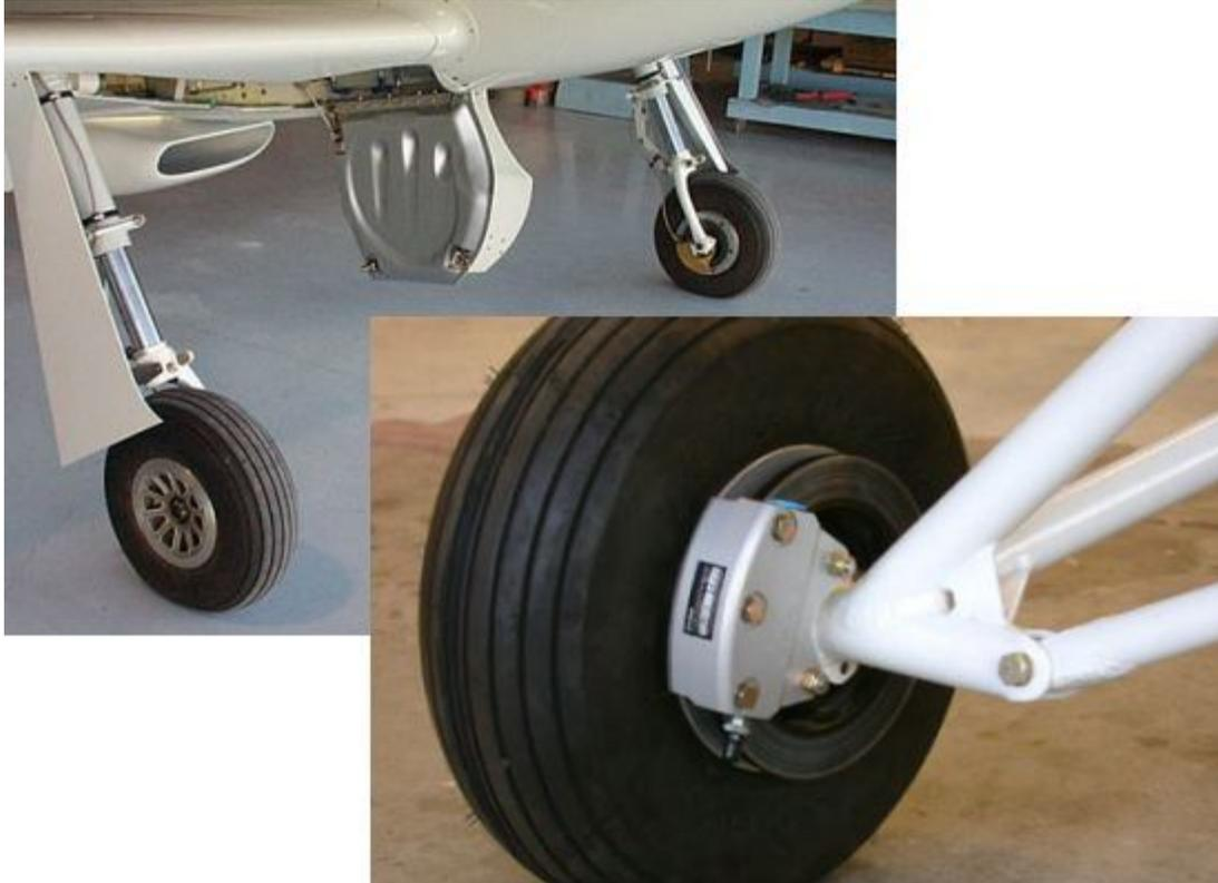
**Wheel brakes used on a typical light airplane**
