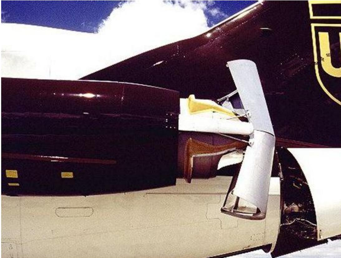
**Clam shell thrust reverser on the DC-9**
