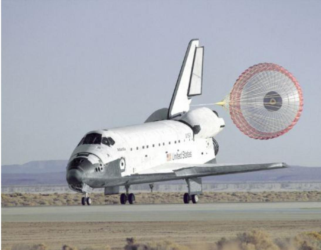
**Braking parachute used on the Space Shuttle**
