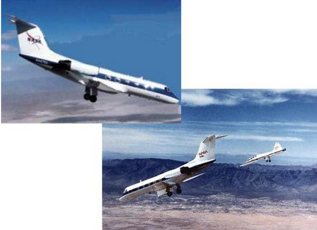
**NASA Shuttle Training Aircraft using thrust reversers**
