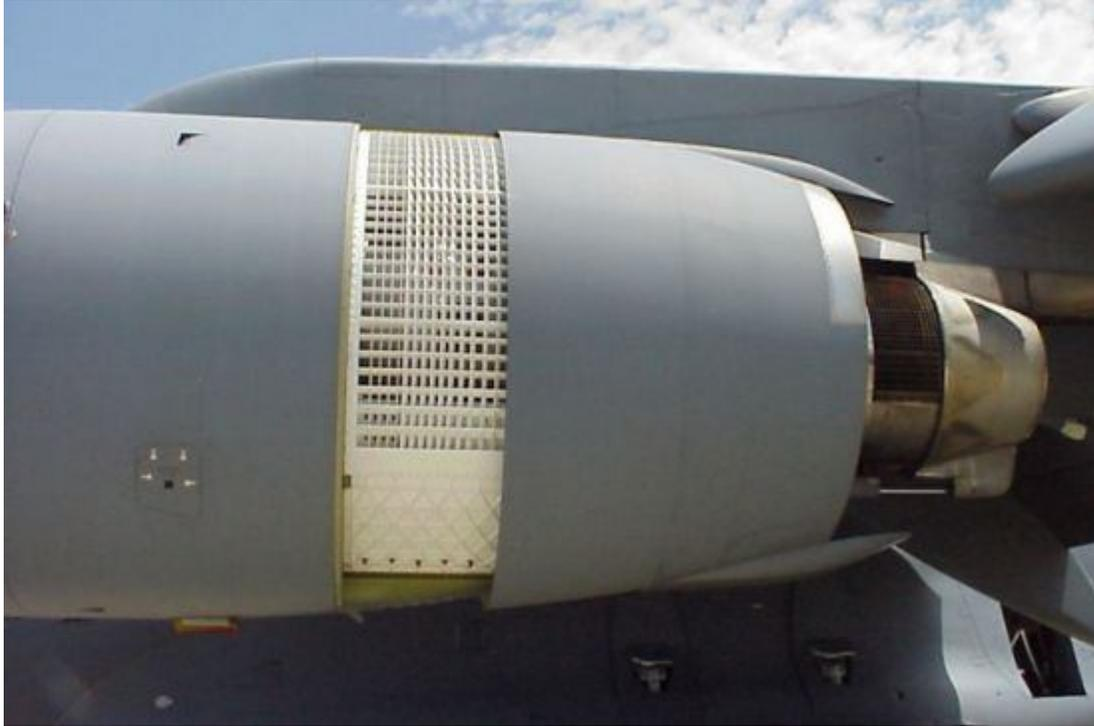
**Cascade thrust reverser on the C-17**
